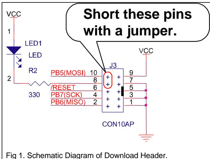
Fig 1. Schematic Diagram of Download Header.
