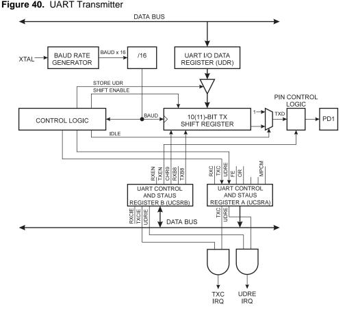
Data transmission is initiated by writing the data to be transmitted to the UART I/O Data Register (UDR). Data is transferred from UDR to the Transmit Shift Register when:
