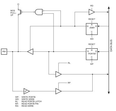
Figure 52. Port B Schematic Diagram (Pin PB2)
