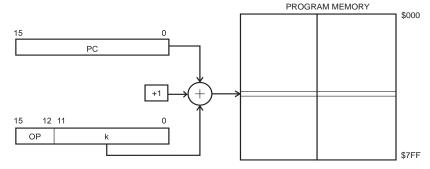
Program execution continues at address PC + k + 1. The relative address k is from -2048 to 2047.
