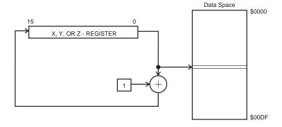
The X-, Y-, or the Z-register is incremented after the operation. Operand address is the content of the X-, Y-, or the Z-register prior to incrementing.
