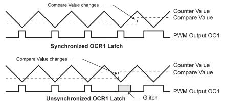
During the time between the write and the latch operation, a read from OCR1 will read the contents of the temporary location. This means that the most recently written value always will read out of OCR1.
