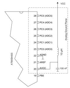
Figure 49. ADC Power Connections
