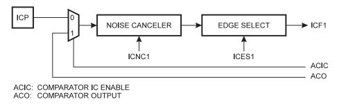
If the Noise Canceler function is enabled, the actual trigger condition for the capture event is monitored over four samples, and all four must be equal to activate the Capture Flag. The input pin signal is sampled at XTAL clock frequency.
