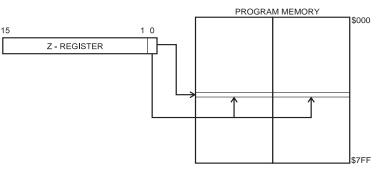
Constant byte address is specified by the Z-register contents. The 15 MSBs select word address (0 - 2K), the LSB selects Low Byte if cleared (LSB = 0) or High Byte if set (LSB = 1).
