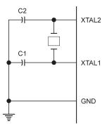
Figure 3. Using MCU Oscillator as a Clock for an External Device
