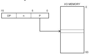
Operand address is contained in six bits of the instruction word. n is the destination or source register address.
