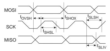
**Table 36.** Serial Programming Characteristics,  $T_A = -40^{\circ}C$  to  $85^{\circ}C$ ,  $V_{CC} = 2.7 - 6.0V$  (unless otherwise noted)
