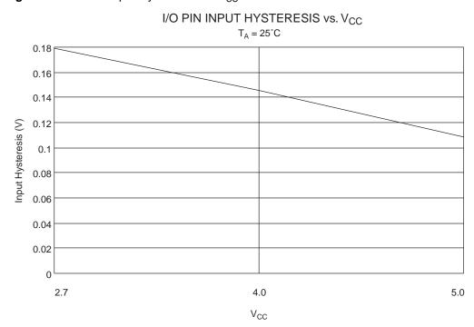
Figure 89. I/O Pin Input Hysteresis vs.  $V_{CC}$
