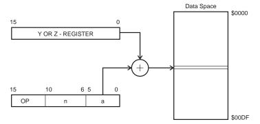
Operand address is the result of the Y- or Z-register contents added to the address contained in six bits of the instruction word.
