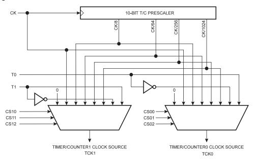
For Timer/Counters0 and 1, the four different prescaled selections are CK/8, CK/64, CK/256, and CK/1024, where CK is the Oscillator clock. For the two Timer/Counters0 and 1, external source and stop can also be selected as clock sources.
