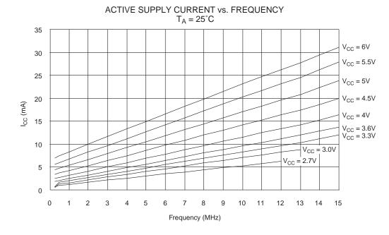
Figure 70. Active Supply Current vs. Frequency
